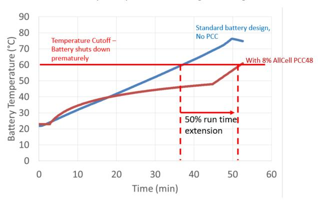
While the blue pack reaches 60 degrees after 36 minutes, the pink pack is able to stay below that cutoff until 52 minutes, resulting in a nearly 50% increase in run time. PCC staves off the high temperatures allowing longer use of high capacity cells even at high power.
